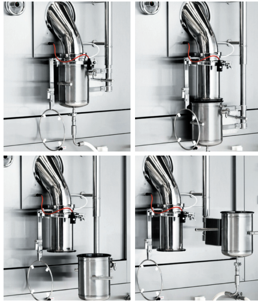
4. Slide and rotate the adapter housing.
